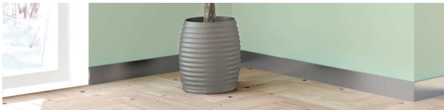
PROSKIRTING LIST is a skirting/baseboard profile in different finishes anodised, polished, brusched, varnished aluminium, 80 mm high and 10 mm wide which can be fixed directly to the wall with adhesive (PKLT .. 80A non-inspectable version) or with aluminum supports (inspectable version PKLT .. 80). The aluminum supports, 20 mm long, are fixed with plugs to the wall, every about 50 cm. PROSKIRTING LIST 80 in aluminum is suitable in any indoor environment.
