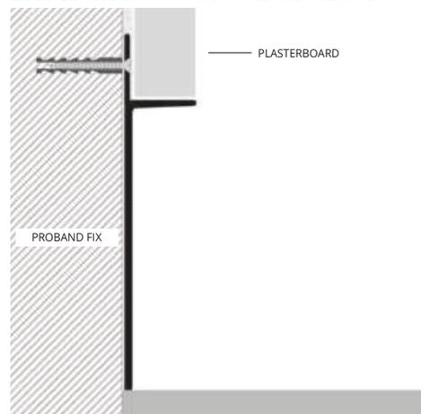
1. Fix "PROSKIRTING INS" using screws (concealed part) and glue/silicone (exposed side), before laying the plasterboard, calculating all the heights and distance. 2. Lay the plasterboard aligning the lower part flush to the "PROSKIRTING INS". 3. Plaster and carry out the surface finishing on the plasterboard.
