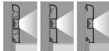
1. Fix the support on the wall putting the screws and plugs every 50 cm (recommended). Make a test with "PROSKIRTING LED" in order to value the height and the correct position of supports.
