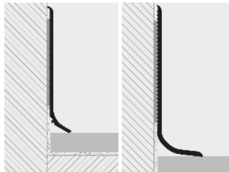
1. Choose the "SKIRTING 60 - 120" of the required height 60/120mm and choose the colour. 2. Lay the "SKIRTING 60 - 120" using an adhesive suitable for gluing flexible PVC onto mortar, plaster, accessorised walls, etc. or fix with screws/nails.
