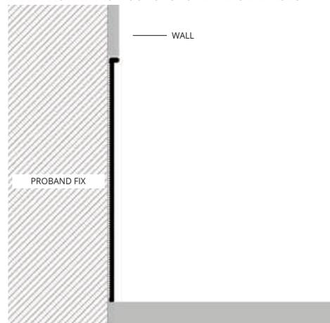
1. Fix the "PROSKIRTING LINE" using glue/silicone (exposed side), before making the required coat, calculating all the heights and distances. 2. Carry out the surface finishing aligning the lower part flush to the "PROSKIRTING LINE".
