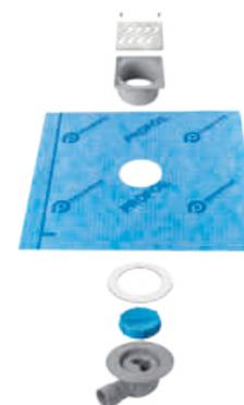
**PROSHOWER DRAIN CENTRAL PRO** is a 10x10 cm stainless steel AISI 316L / 1.4404 – V4A drain for the realisation of floor-level shower. This low thickness drain is equipped with a grid that can also be tiled for floor-level drains. PROSHOWER DRAIN CENTRAL PRO has excellent chemical resistance and is equipped with a 360 ° adjustable siphon.
