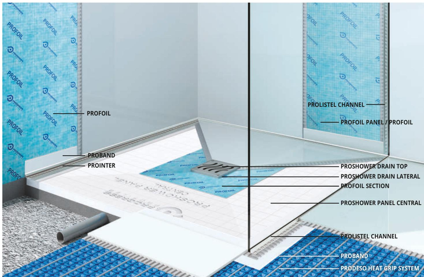
**PROSHOWER LATERAL DRAIN KIT** are 2 central drain systems with lateral outflow equipped with a siphon, grate support, stainless steel grate, butyl double-sided ring for the fixing of the waterproof section, waterproof section and a protection cap with template function too that allows the correct positioning of the butyl ring and the waterproof section. LATERAL AND VERTICAL DRAIN KIT ensure a correct flow of rainwater.
