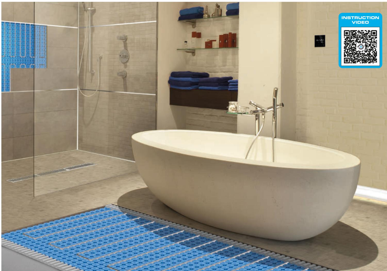
Uncoupling and waterproofing membrane in polypropylene with a thickness of 5.5 mm. The membrane is provided on top with pseudo-square reliefs which create channels for fixing the electric heating cable. On the back of the membrane there is a layer of adhesive which guarantees its fixing to the support, clean plywood, OSB, metal or old flooring.
