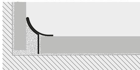
1. Choose "PROINTER KL ACC" according to the desired finish. 2. Cut "PROINTER KL ACC" to the desired length. 3. Apply the silicone along the floor-wall connection. 4. Press the arrowhead of "PROINTER KL ACC" into the silicone evenly until it is completely adherent to the floor and wall.
