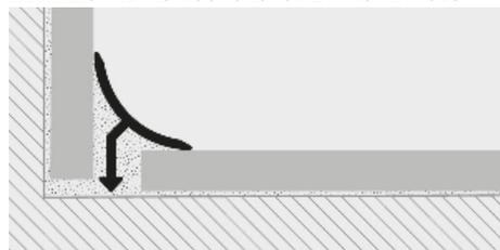
1. Choose "PROINTER KL ALL" according to the desired finish. 2. Cut "PROINTER KL ALL" to the desired length. 3. Apply the silicone along the floor-wall connection. 4. Press the arrowhead of "PROINTER KL ALL" into the silicone evenly until it is completely adherent to the floor and wall.
