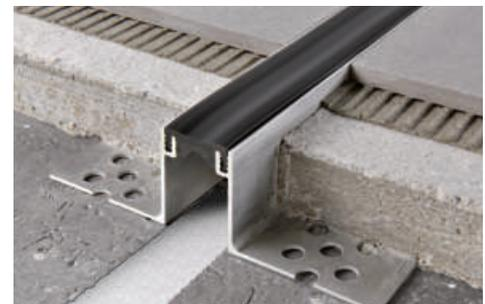
1. Choose the colour of the joint. 2. Fix the punched flanges to the substrate using screws and screw anchors, calculating the fixing points at 30cm intervals on both sides. 3. Make the screed over the punched flanges of the structural or expansion joint, calculating the thickness of the final floor, and then lay the floor as normal. 4. Using the special glue, fill the gap between the tiles and the profile.
