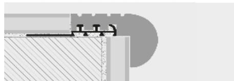
1. Choose the PROSTAIR WOOD Z with suitable height for the thickness of the covering of the step or staircase.
