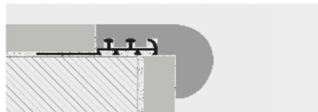
1. Choose the PROSTAIR WOOD with suitable height for the thickness of the covering of the step or staircase.
