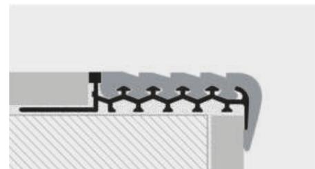
1. Choose a PROSTAIR 50 height and color corresponding to the thickness of the tile. 2. Fix the riser laying it at the appropriate and definitive height. 3. Fill the empty spaces under the square completely with adhesive. 4. Rest the adhesive on the tread, lay the square with the base cut in the adhesive and line it up so that the square covers the tile edge of the riser. 5. Lay the tiles of the tread lining them up with upper part of the square so that it meets with the edge.
