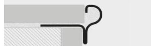
1. Choose the PROSTYLE with suitable height for the thickness of the floor (stairs). 2. Apply the adhesive onto the area of application of the profile. 3. Lay and align the profile, cut to the necessary length, pressing the perforated flange into the adhesive. 4. Lay the tiles, aligning them so that the top edge of the profile is "flush" with the tile. 5. Fill the profile/tile area of contact with adhesive to prevent the accumulation of water in any voids.
