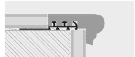
1. Choose the PROSTYLE WOOD with suitable height for the thickness of the covering of the step or staircase. 2. Apply the adhesive onto the area of application of the profile. 3. Lay and align the profile, cut to the necessary length, pressing the perforated flange into the adhesive. 4. Lay the step covering, aligning it so that the top edge of the profile is "flush" with the covering. 5. Fill the profile/covering area of contact with adhesive to prevent any infiltration.
