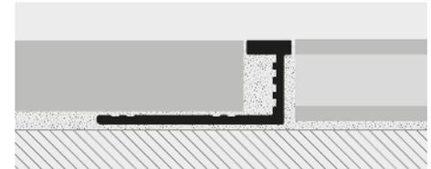
1. Choose the "PROELEGANT CURVE" in the required height and material. 2. Cut the profile to the necessary length, calculating the total length. 3. Bend the profile mechanically with the PROCURVE MACHINE. 4. If necessary fix with screws and screw anchors or simply insert the punched base under the floor laid with the same adhesive. Any oxidation marks may be easily removed with specific chemical products (Sidel-Smac, etc.).
