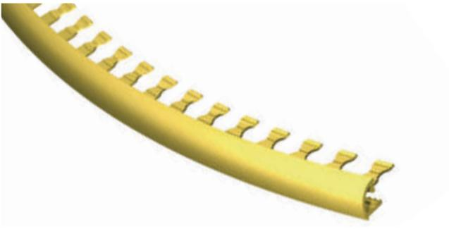
**PROJOLLY CURVE** is a range of terminal transition profiles that may be curved/shaped, with a special system of perforations allowing it to be bent so that particular geometric shapes may be easily obtained in situ. This allows decorative patterns to be created at will according to technical and aesthetic requirements. It is made in anodized aluminium, height H 8 - H 10mm, length 2.7 lm.
