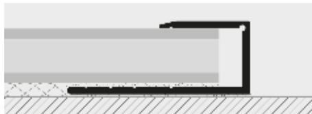
1. Choose the "TERMINAL CURVE" in the required height and material. 2. Cut the profile to the necessary length, calculating the total length. 3. Bend the profile mechanically with the PROCURVE MACHINE. 4. If necessary fix with screws and screw anchors or simply insert the punched base under the floor laid with the same adhesive.
