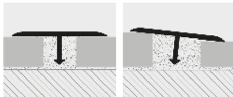
1. Choose the "PROCOVER" with the width suitable for the gap between the two floors to be joined, taking into consideration 2/3 mm side lap. 2. Fill the gap with single-pack silicone or with the adhesive used for laying the floor. 3. Bury the profile into the adhesive, making sure that both side laps of the profile rest on the coverings to be joined.
