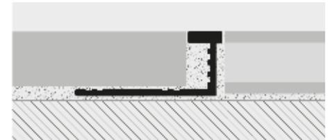
1. Choose the "PROELEGANT CURVE" in the required height and material. 2. Cut the profile to the necessary length, calculating the total length. 3. Bend the profile mechanically with the PROCURVE MACHINE. 4. If necessary fix with screws and screw anchors or simply insert the punched base under the floor laid with the same adhesive. Any oxidation marks may be easily removed with specific chemical products (Sidel-Smac, etc.).
