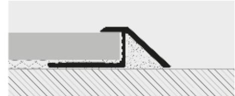
**PROSLIDER CURVE** is a range of transition profiles that may be curved/shaped, with a special system of perforations allowing it to be bent so that particular geometric shapes may be easily obtained in situ. This allows decorative patterns to be created at will according to technical and aesthetic requirements. Recommended for joining floating floors in wood, melamine laminated wood and ceramics. It is made in anodized aluminium in various heights, length 2.7 lm.
